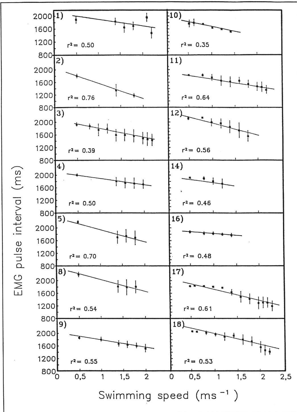
**Figure 2.** Calibration of EMG pulse intervals to swimming speed in individual Atlantic salmon by use of implanted EMG radio transmitters. The markers (with standard deviations) represent an EMG average at each swimming speed. (Decreased EMG pulse intervals indicate increased muscle activity.)
